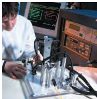
▲ AUTOMATIC CONTINUITY & INSULATION RESISTANCE TEST
